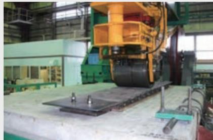
Wheel load running test
