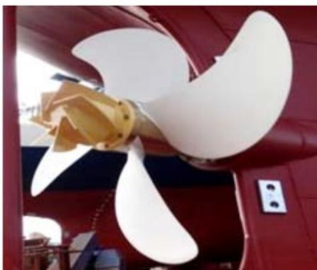
Propeller made with carbon fiber
