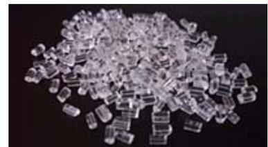
DURABIO™ is a polymer that is made from isosorbide, which is derived from saccharides, a plant-based material.
