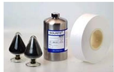
Four key materials (from left: cathode material, anode material, electrolyte, and separator)
