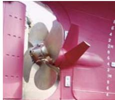
Fins added to ships to increase fuel efficiency
