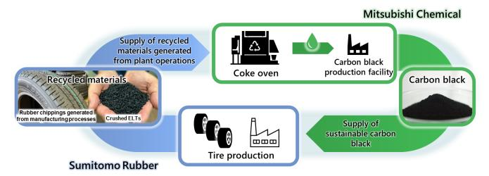
According to the collaboration plan, Sumitomo Rubber will supply rubber chippings (recycled materials) generated from tire manufacturing processes and crushed end-of-life tires ("ELTs") to Mitsubishi Chemical. At Mitsubishi Chemical, these materials will be fed into coke ovens as raw materials for chemical recycling\*1 to produce carbon black again from the tar. The resulting sustainable carbon black will be used as raw material for tires to be produced by Sumitomo Rubber.
